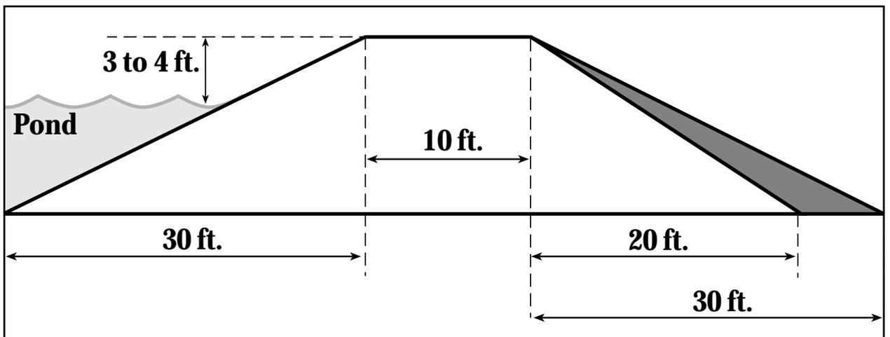
wide for each foot of dam height. A 3:1 slope is much easier and safer to mow than a 2:1 slope, but it will increase construction costs.
