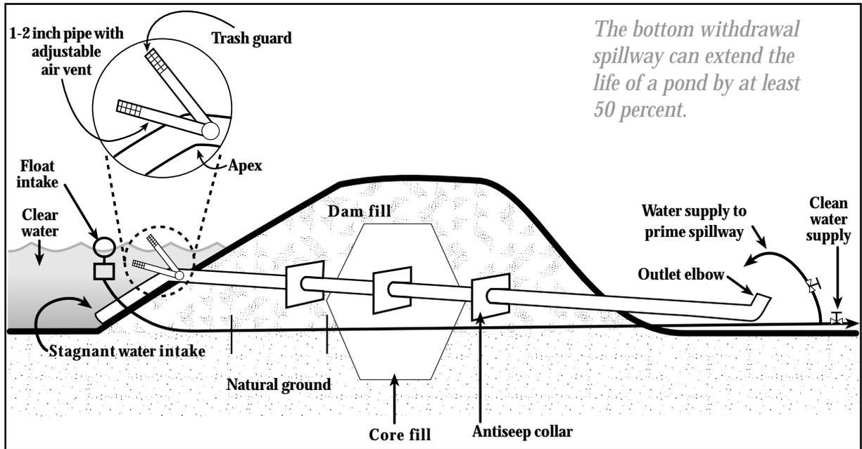
12 inches below the earthen spillway level to keep water from flowing across the earthen spillway. Constant water flow over the earthen spillway will leave it moist and vulnerable to severe erosion during heavy rains. The trickle tube should be large enough to carry most runoff, or just large enough to draw the water level down in a short period of time after water quits flowing in the pond.
