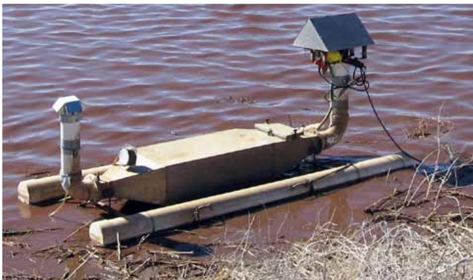
*Figure 4. A wind tunnel floating on the surface of a runoff retention structure collects air samples, which are sent to a hydrogen sulfide analyzer. (Photo: K. Casey)*
