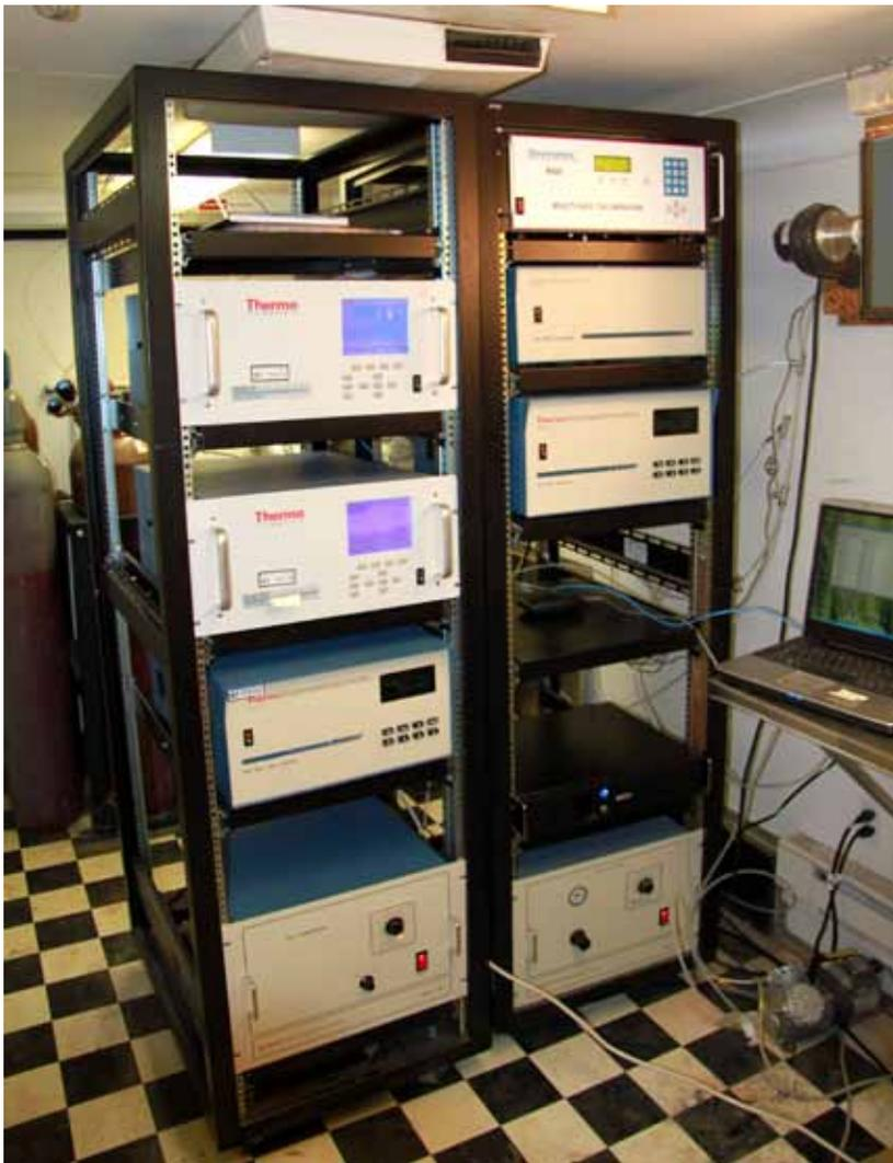
*Figure 2. Several gas analyzers operating inside a trailer deployed at a concentrated animal feeding operation including two hydrogen sulfide analyzers (Model 450i, left rack, second from top; Model 45C, left rack, third from top) by Fisher Scientific (Waltham, MA). (Photo: K. Casey)*
