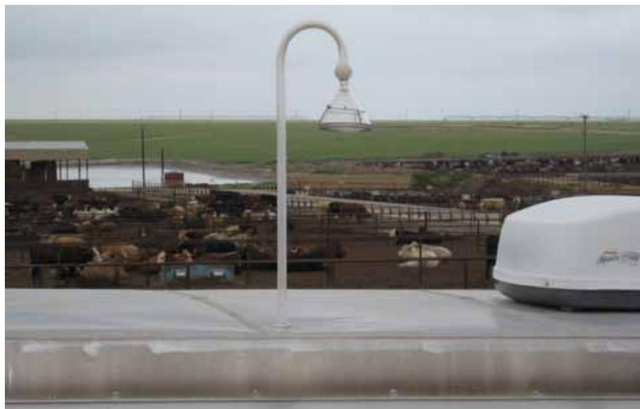
*Figure 3. An intake port mounted on the roof of a trailer deployed at a concentrated animal feeding operation provides air samples to hydrogen sulfide analyzers inside the trailer. The pen surfaces and runoff retention structure visible in the background are potential sources of hydrogen sulfide. (Photo: K. Casey)*
