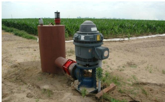
Figure 3. Wellhead irrigation pump (Photo: USDA)
