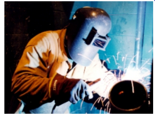
Figure 3.3.c. Welding produces fumes. As the metal melts, and the welding rod and flux covering is burned, fumes are produced. These fumes can cause irritation to the nose and lungs.
