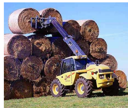
Figure 3.1.f. Hydraulic systems often have stored energy.
