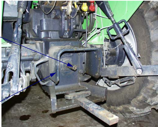
Figure 3.1.b. A PTO stub and a master shield on a tractor. A PTO is a wrap point hazard that causes countless injuries and deaths each year.
