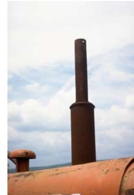
Figure 3.2.a. A straight pipe used for the exhaust or a worn-out muffler will increase noise levels coming from the engine. Muffler condition should be part of a safety audit.
