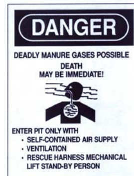
Figure 3.3.1.a. Safety signs warn us of immediate danger. This sign tells us that respiratory protection is required. What other safety practices does this warning sign recommend?
