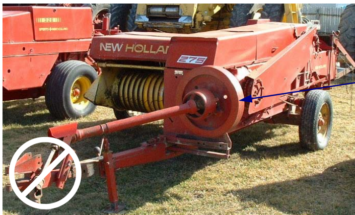
Figure 3.1.d. The flywheel on a small square baler is an example of a freewheeling part. The flywheel keeps the baler running smoothly if a large amount of hay is suddenly taken into the bale chamber. Notice that part of the PTO driveline is unguarded.
