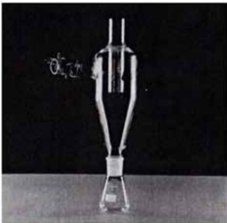
**Aerojet® cyclone sampler**
