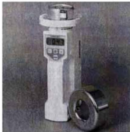
**RSC Biotest® centrifugal sampler**
