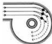
2. Centrifugal inertial impaction: particle separation by centrifugal force in a radial geometry (Reuter centrifugal sampler, BIO)
