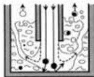
3. Liquid impingement: the particles are collected by inertial impaction into a liquid, and particle diffusion within the bubbles (the AGI-4 and AGI-30 impingers)
