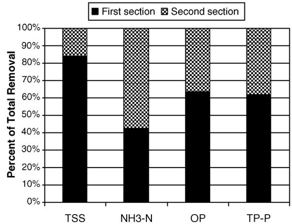
Fig. 5. Removal contributions by section during normal operations.
