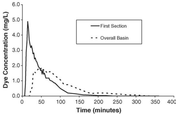
Fig. 3. Tracer dye concentrations vs. time, Aquamats<sup>®</sup> removed.
