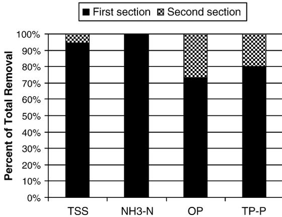
Fig. 4. Removal contributions by section during cleaning and harvesting activities.
