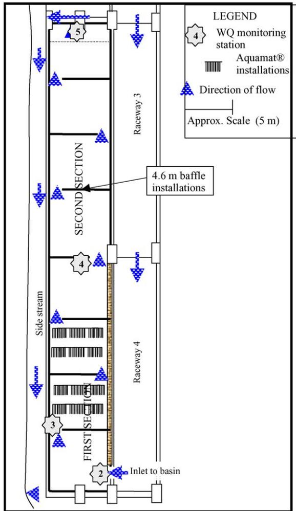
Fig. 1. Plan view of raceways and sedimentation basin.
