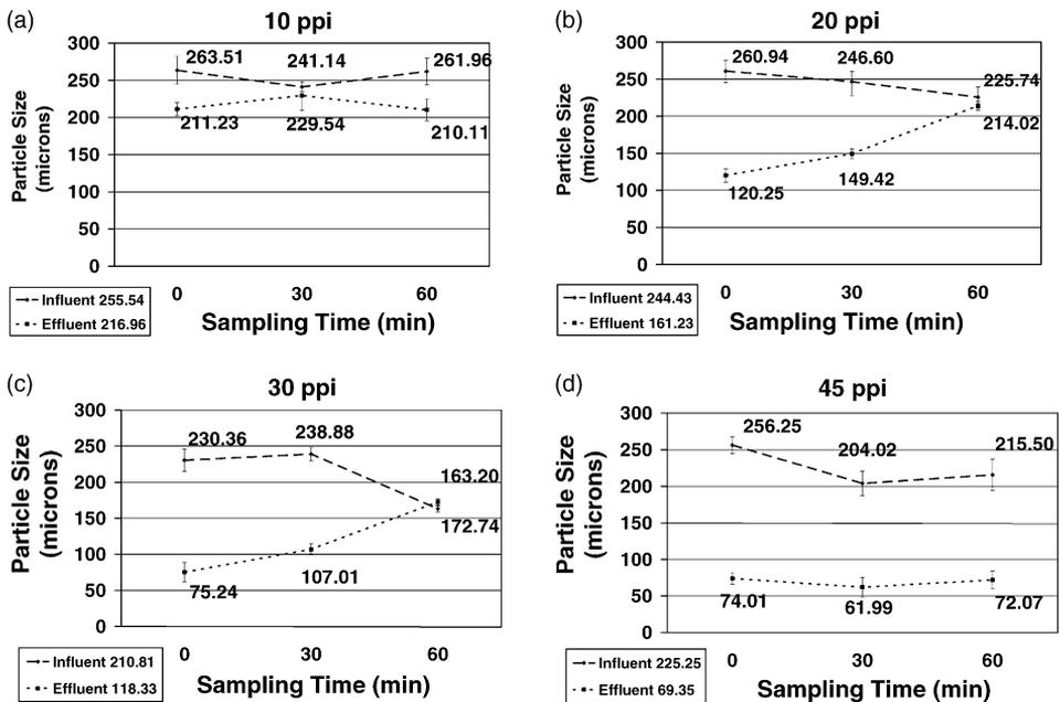
Fig. 2. Bench top influent and effluent particle size for (a) 10 ppi (b) 20 ppi (c) 30 ppi and (d) 45 ppi reticulated foams. Note: Test averages shown in the legend.
