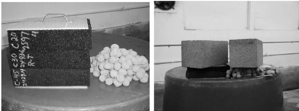
Fig. 1. Reticulated foam (to the left in each picture) and Fuzzy filter<sup>®</sup> media (to the right in each picture) in the uncompressed and compressed states, left picture and right picture, respectively.
