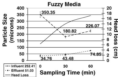
Fig. 4. Bench top influent and effluent particle size for Fuzzy media. Note: Only the Fuzzy media had measurable head loss.
