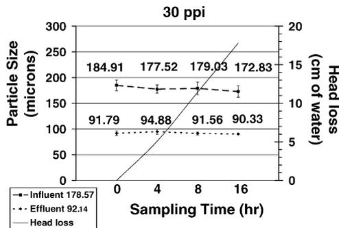
Fig. 5. Particle capture and head loss field test results for 30 ppi reticulated foam filtration trial. Note: Test averages shown in the legend.
