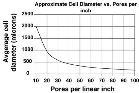
Fig. 3. Average cell diameter as a function of Foamex<sup>®</sup> reticulated foams. Data taken from Foamex<sup>®</sup> technical product function sheet.
