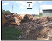
4 Condense windrow into conical shape.
